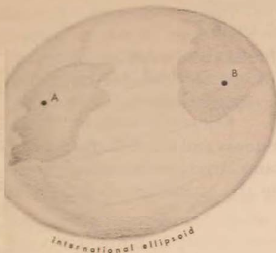
2. Corrected points are transferred onto the international ellipsoid.
